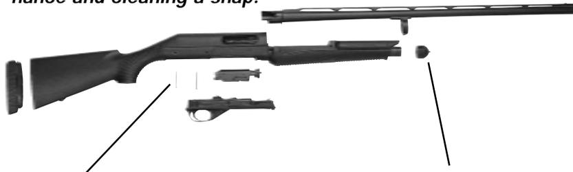
*Two easily removed pins permit removing the trigger group for cleaning. The forend nut is the tool to remove the pins. The "checkering" worked very well.*
