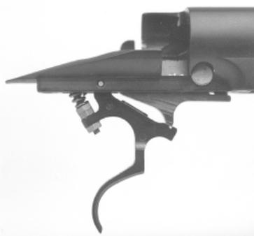
*The Winchester's trigger broke crisply at 4.5 to 4.75 pounds and showed a little creep. To adjust this trigger, the pieces would have to be broken down and honed to get a lighter, smoother pull. That's a job for a gunsmith.*
