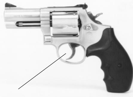
not pull back the hammer? The first sign of a problem was a loss of trigger return. Attempts at firing single action resulted in getting the hammer to drop but not with sufficient force to detonate the rounds. It's ironic that such a heavily built gun wouldn't tolerate more than 10 shots of PMC's 180-grain jacketed hollow point.
