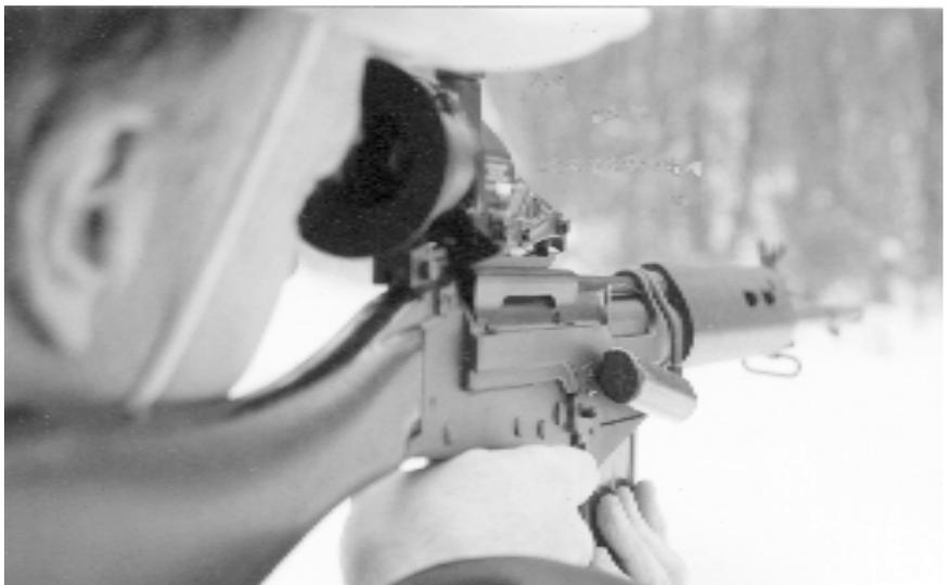
*The L1A1 shines in any weather with its SUIT scope. The SUIT, or Trilux, or L2A2 scope is today sold without the original green radiating element that illuminated the reticle. However, a battery unit is available to light the inverted post red, for better visibility in marginal light. This efficient combination rated very close to the M1A in our tests. This one is built on the Enterprise receiver.*
