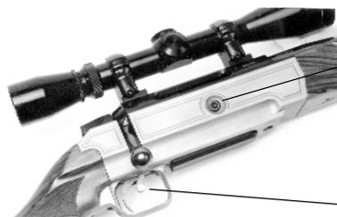
The Jewell benchrest trigger adjusts down to 6 ounces. We liked the position of the safety inside the trigger guard.
