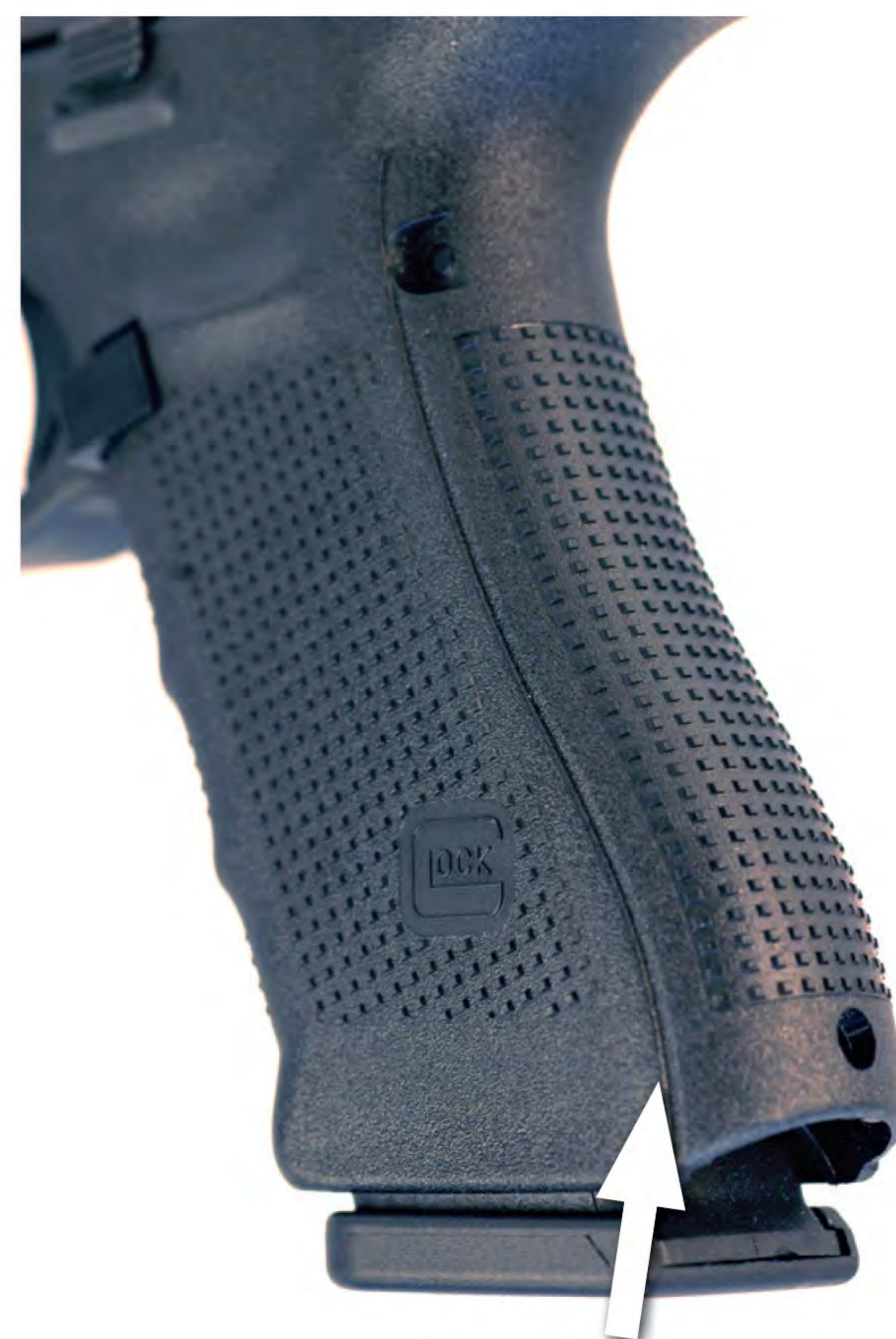
Right: The new texture, also found on the RTF models, looked more abrasive than it actually was. It helped us hold on in hot weather, but we found it was most beneficial when shooting with gloves on, such as many patrolmen wear. Note the vertical ridge at the rear corner of the grip. That's not just to create the illusion of a side panel. That groove holds the alternate backstraps in place.
