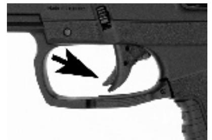
Right: The trigger face included a safety much like the Glock design. Testing the PPS at 12 yards proved that the Walther was accurate and easy to shoot.
