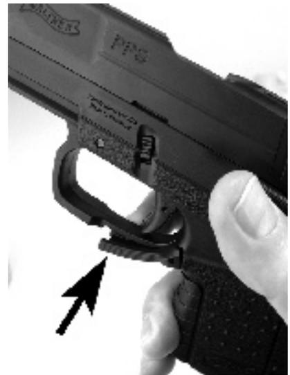
The magazine release was integrated with trigger guard. We liked to operate it with the middle finger.
