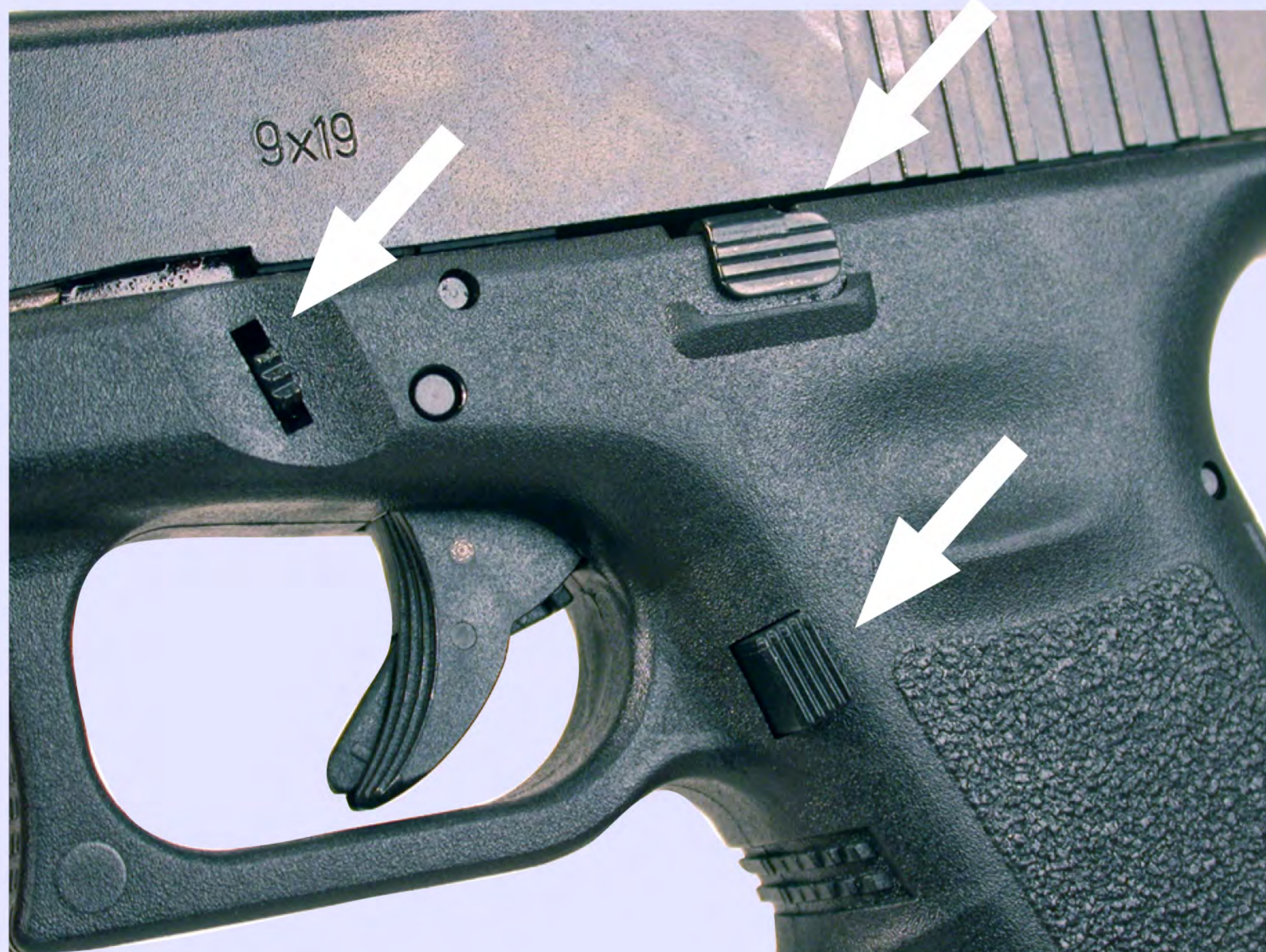
Above: The magazine release (bottom arrow), takedown levers (left arrow), and the slide release (right arrow) were the only manual controls aside from the trigger. Despite them being mounted tightly against the frame, we found all three levers were accessible.
